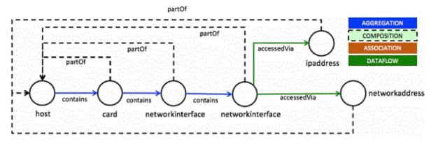
The partOf relationship is not shown as an explicit edge in the toplogy UI. However, it is used to determine which resources should be hidden in the host-to-host view, which in the context of this scenario would show just the hosts 172.20.1.104 and 172.20.1.1, as well as the connectedTo edge between them, as depicted in the following part of the image.
