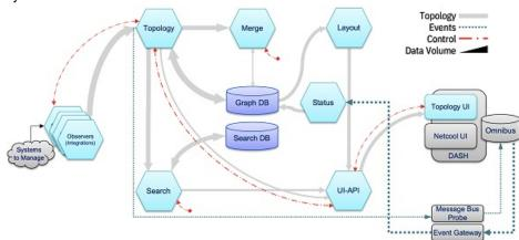
Specifically, this diagram shows how the data flow from Agile Service Manager status generates Netcool/OMNIbus events. When Netcool/OMNIbus is the source of events, however, the data flow from the Event Observer to the topology service not only updates the status eventId with ServerName/ServerSerial, but generates the status itself.
